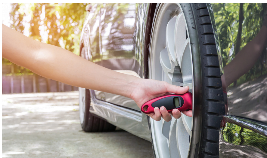
AIR SUPPLY – AAA recommends regularly using a tire gauge to monitor tire pressure. Image: NongAsimo. Adobe Stock.
